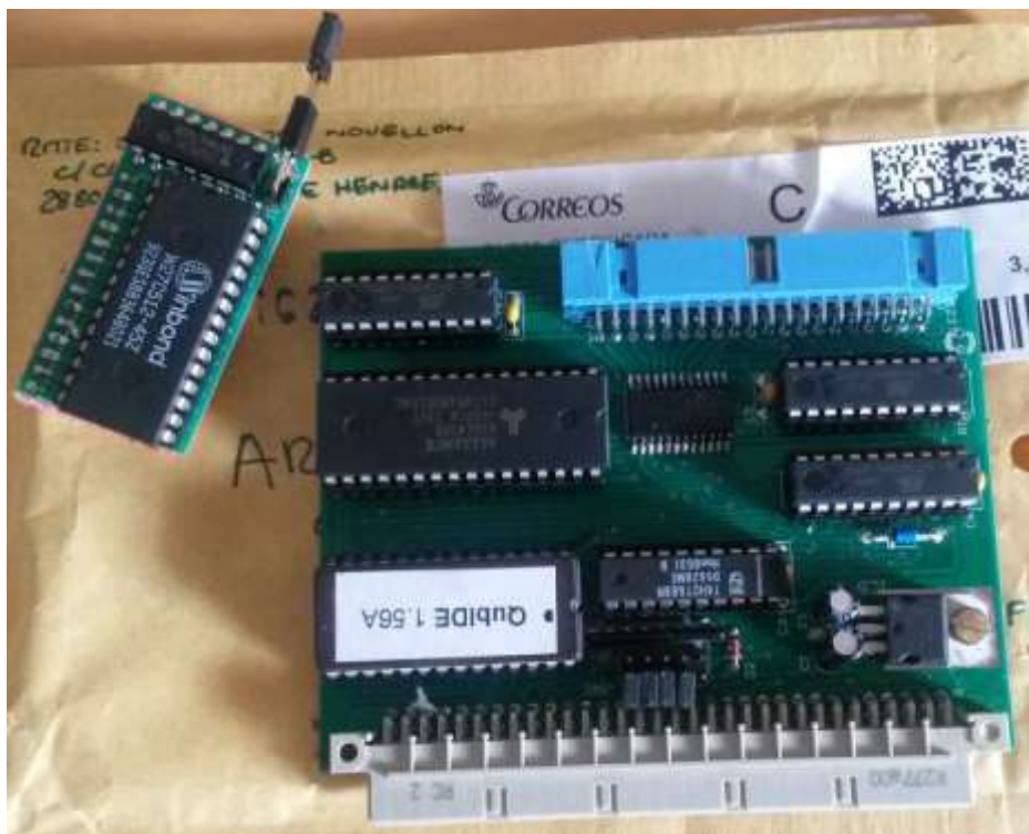
QubIDE with firmware version 1.56A
